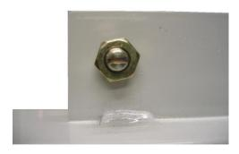
Using the slot as a guide, turn the screw one complete turn clockwise. This will space the profile off the corner 1.5mm. If you prefer a greater spacing, each half turn will give 0.75mm clearance. It is VERY important that both setting screws are set to the same distance.
