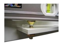
Slacken the lock nut on the screw to be adjusted and place the Profile on a flat surface with the wobbly foot facing upwards. Place a spirit level or other straight edge diagonally over the profile stalk and the foot of the setting screw to be adjusted as shown above.
