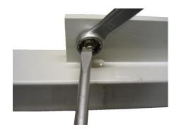
Hold the setting screw with a screwdriver to prevent it turning and pinch the lock nut with a spanner to preserve the adjustment. Repeat the adjustment for the second screw.
