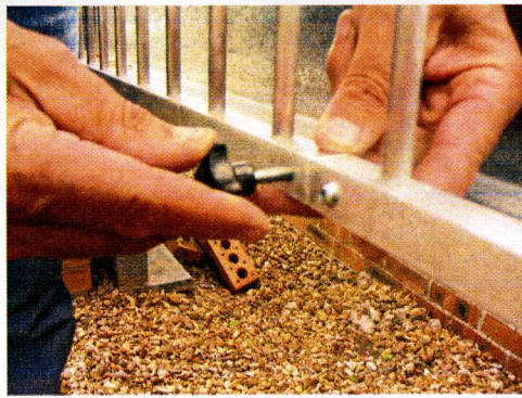
Securing ladder sections
